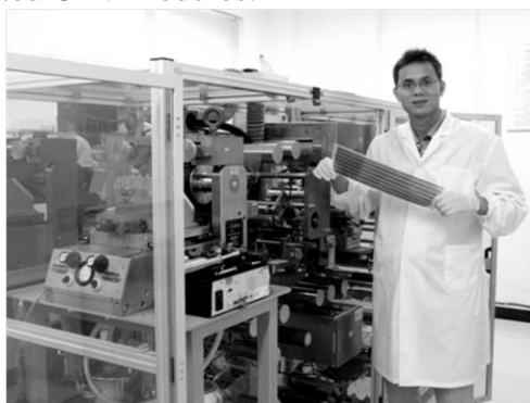
Fig.1 Self-developed R2R multi-function printer/coater and its application in the fabrication of organic solar cells
