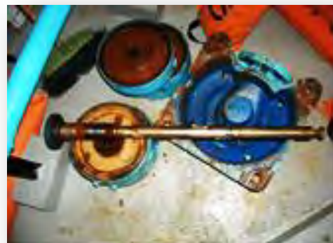
Defective water pump motor bearings renewed
