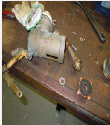
2" water filling ball valve of Floor 3, AM Building fresh water tank reconditioned
