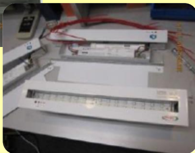
Failed LED light stripes of 285 nos. of EXIT light boxes at AC1, CYC Building, FYW Building, MMW Building public corridors were replaced, instead of replacing the whole EXT light boxes
