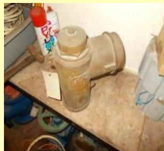
Flush water ball filling valve of the basement flush water tank at SC21, AC1 was re-conditioned
