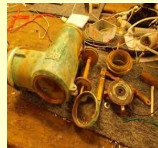
Flush water ball filling valve of the basement flush water tank at SC21, AC1 was re-conditioned
