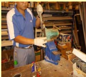
Flush water ball filling valve of the basement flush water tank at SC21, AC1 was re-conditioned
