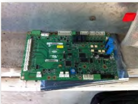
Defective electronic control cards instead of replacement by OEM were repaired
